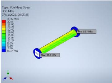
Factor of safety come as 8.19, according to the regulations it needs to be more than 4.5 for the oil and gas industry. The displacement and Von Mises stresses also have been generated. The extended report will be given to your company as an attachment.
